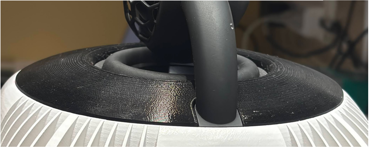
Figure 48 DM Cover Properly Installed
