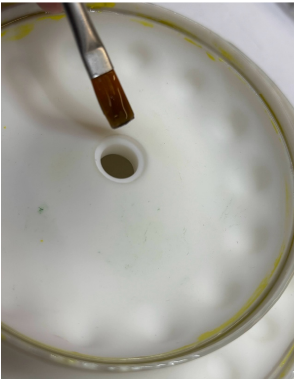
Figure 27 Base Center Hole Bonding
