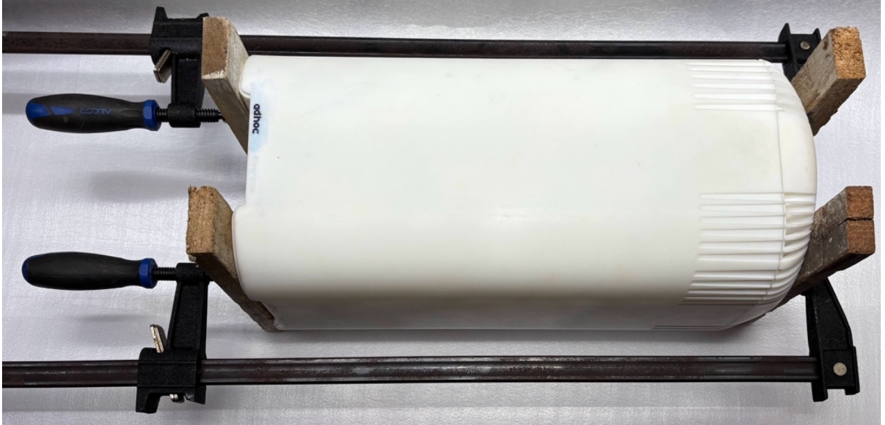
Figure 28 Clamping The Enclosure Parts For Curing
