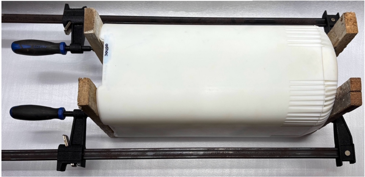
Figure 15. Clamp the Enclosure parts for curing
