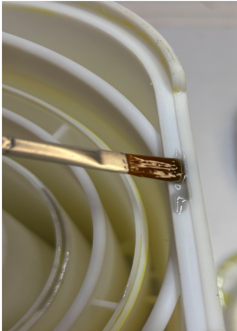
Figure 13. Tube Section-to-Base epoxy/adhesive areas.
